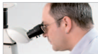
The viewing angle is adjustable from 5°–45° for the most relaxed head position possible
